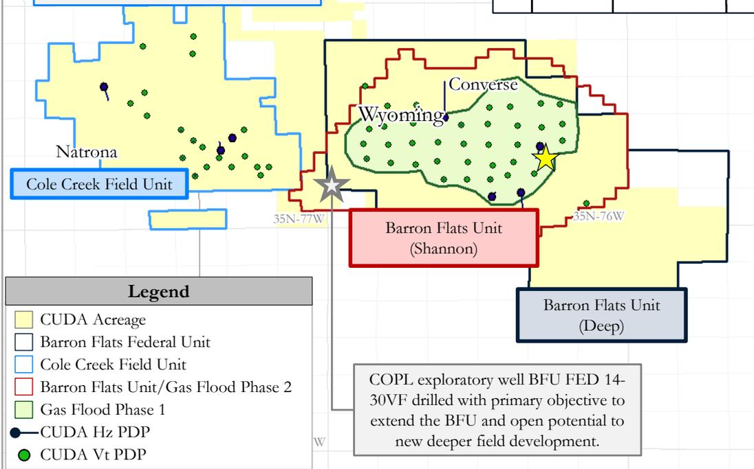
COPL exploratory well BFU FED 14-30VF drilled with primary objective to extend the BFU and open potential to new deeper field development.
